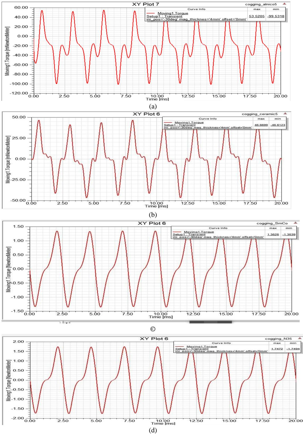
**Figure2. Cogging torque of BLDC motor for different types of four magnet materials: (a)Alnico5(b)ceramic 5(c)sms028(d) NdFe 35**
