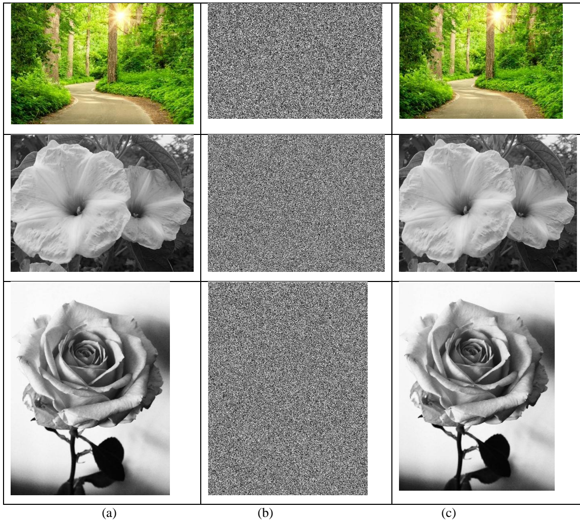
Figure 11: The simulation results of a cryptosystem CSS: (a) grayscale and Color plain images; (b) cipher images of (a); (c) decryption of (b)
