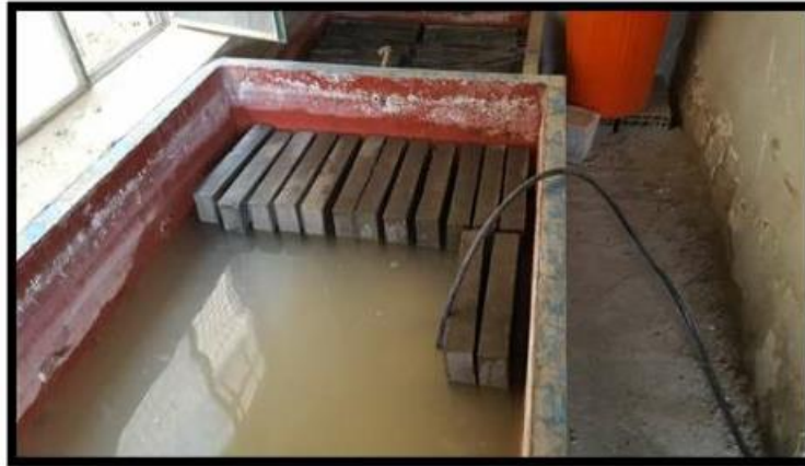
Figure 6. Slabs during curing.
