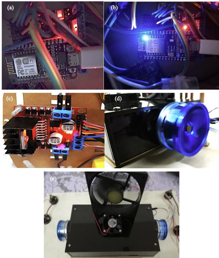
Figure 7, (a) Indicator of the system turned ON, (b) the Indicator of the Wi-Fi Module Connected, (c) the motor driver connected to Arduino, (d) the motor working with adjustable speed, and (e) Other load functions.
