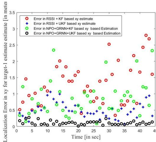
Figure 8: Localization errors in x-y estimates for target 1 in RSSI+KF, RSSI+UKF, and proposed methods
