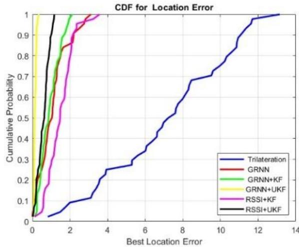
Figure 11: CDF of the location errors based on the Trilateration, GRNN, GRNN +KF, GRNN +UKF, RSSI+KF, and RSSI+UKF for target 2
