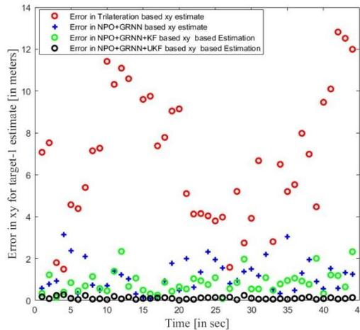
Figure 6: Localization errors in x-y estimates for target 1 in Trad RSSI and proposed methods
