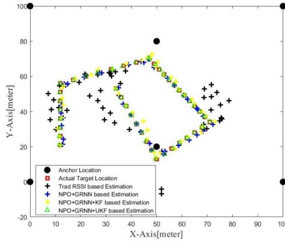
Figure 5: Actual and target estimated for target 2 by Trad RSSI and proposed methods
