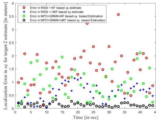
Figure 9: Localization errors in x-y estimates for target 2 in RSSI+KF, RSSI+UKF, and proposed methods
