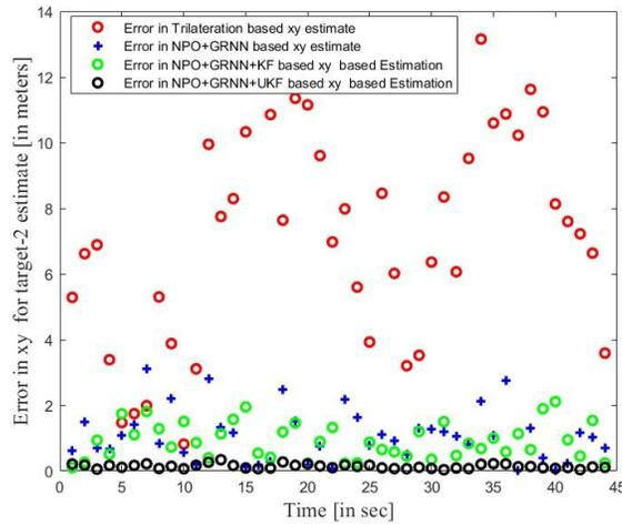
Figure 7: Localization errors in x-y estimates for target 2 in Trad RSSI and proposed methods
