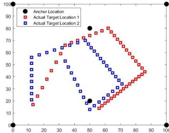
Figure 3: Actual two target Locations and 6 anchor nodes
