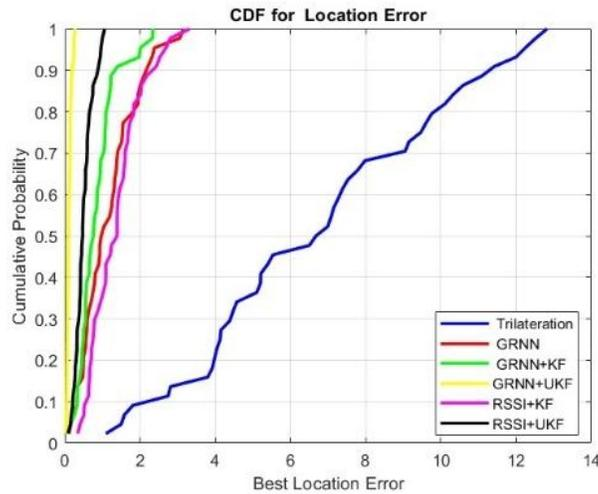
Figure 10: CDF of the location errors based on the Trilateration, GRNN, GRNN +KF, GRNN +UKF, RSSI+KF, and RSSI+UKF for target 1
