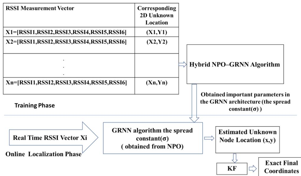
Figure 2: The hybrid NPO-GRNN-KF algorithm's block diagram
