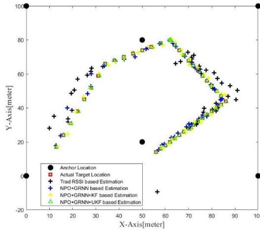
Figure 4: Actual and target estimated for target 1 by Trad RSSI and proposed methods
