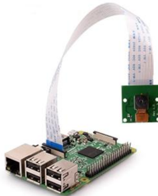
Figure 3, The connection between Raspberry Pi 3 board and Camera Model
