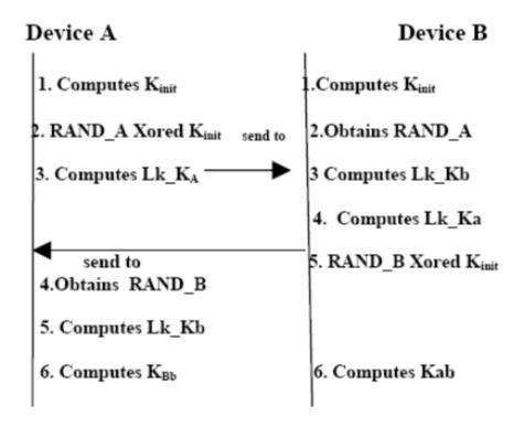
Fig. (4) Bluetooth coupling Mechanism
