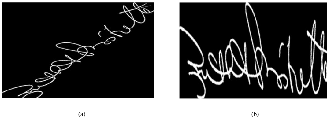
Figure 5. Rotation Compensation Step Results :( a) The Image Before Applying Rotation Compensation, (b) The Image After Applying Rotation Compensation
