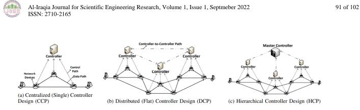
Figure 2: An overview of the most common SDN control plane [25].
